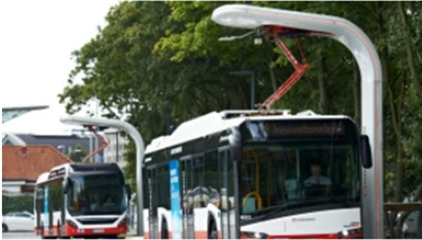
FIGURE 72: TOP-DOWN PANTOGRAPH IN HAMBURG. SOURCE: (Siemens, 2018)
