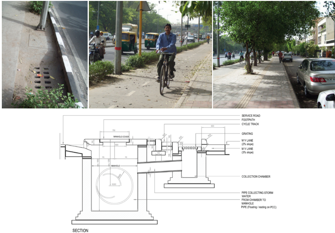
Figure 36 : Drainage for arterial streets (Source : SGArchitects, Delhi)
