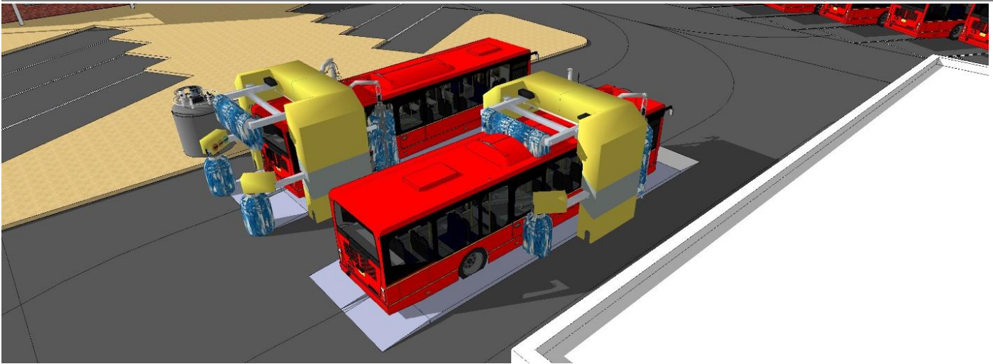
Figure 44: View of washing area showing gantry washers
