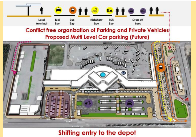
Figure 65: Proposed depot, Local terminal area and Private parking area (same for both proposals)
