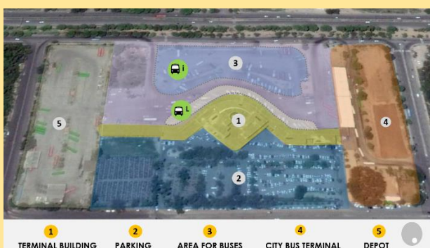
Figure 62: Components of existing terminal
