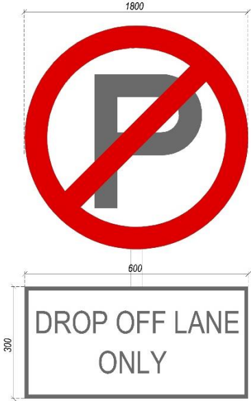
REGULATORY SIGN : DROP OFF LANES
