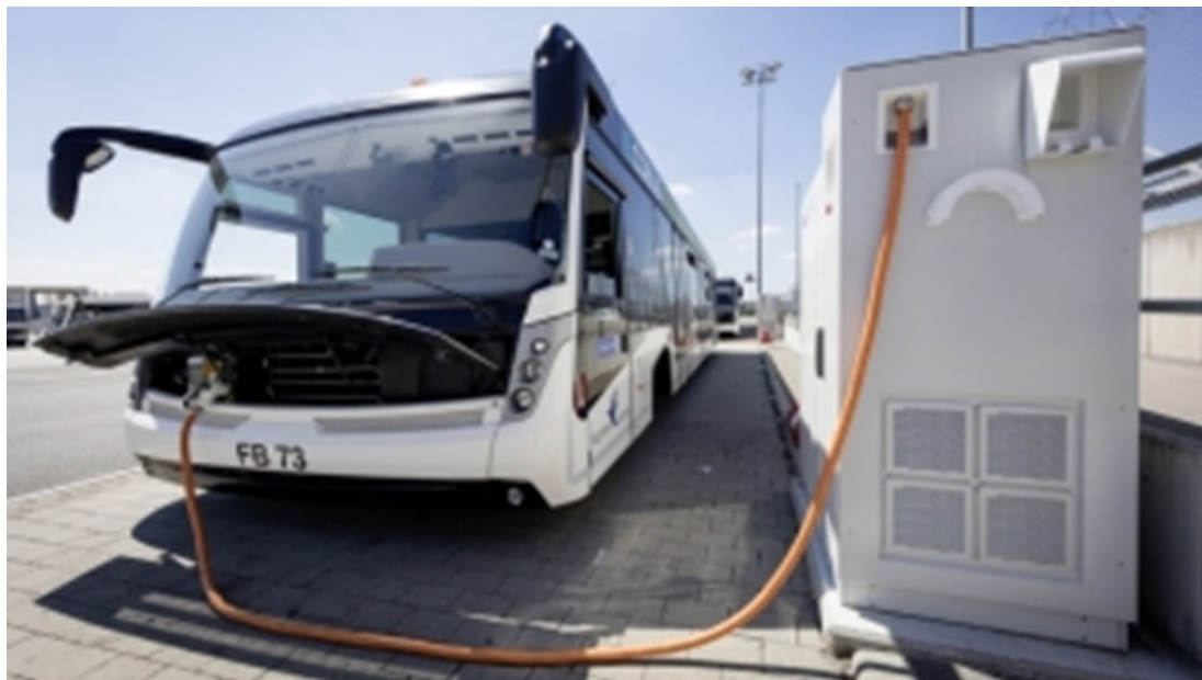
FIGURE 71: PLUG-IN CHARGING AT THE AIRPORT STUTTGART. SOURCE: (Siemens, 2018)
